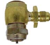
9044 Lock Chuck (Standard Bore) .307-32 thread and .375-24 side hose connector. Maximum operating pressure of 3000 PSI
