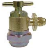
8927 Lock Chuck (Large Bore) T-Handle with .485-26 thread and .375-24 side hose connector. Maximum operating pressure of 3000 PSI
